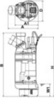
W1: lowest running water level
