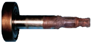
304 stainless steel cast impeller was mounted on 403 stainless steel shaft. ( Shaft was heavily corroded )
